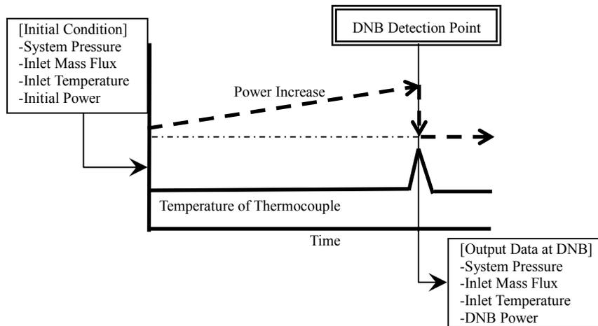
**Figure 3 Schematic drawing of test parameter behavior**
