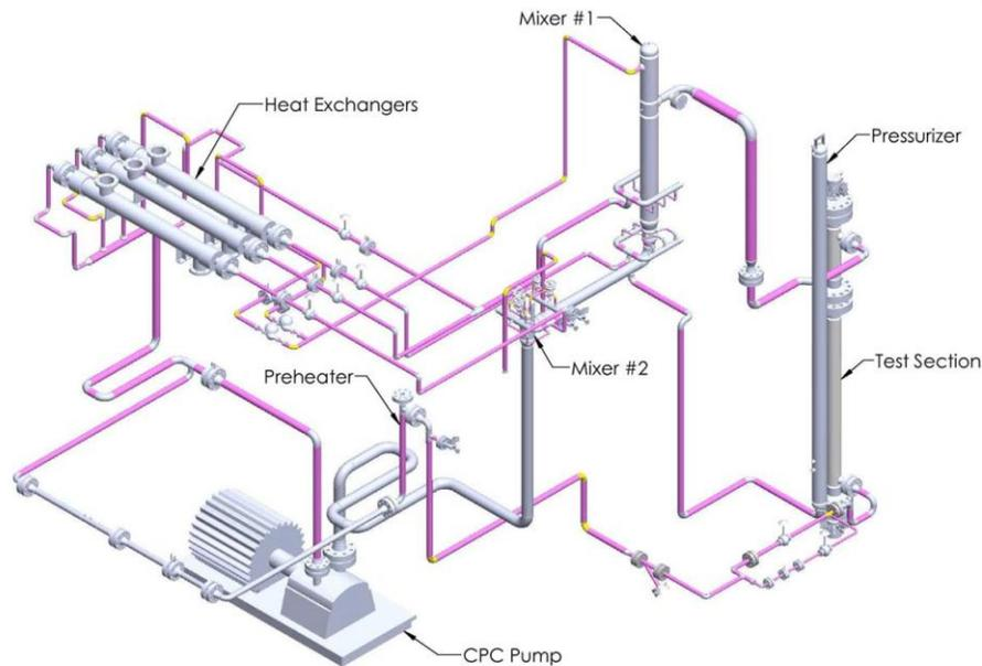
**Figure 1 Isometric view of SL Test Loop**
